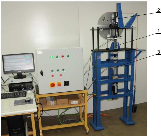
Fig. 4. The view of the apparatus built by the Institute for Sustainable Technology, Radom with mounted cylindrical tribotester (1), loading pulley (2), normal load and torque indicators (3)
