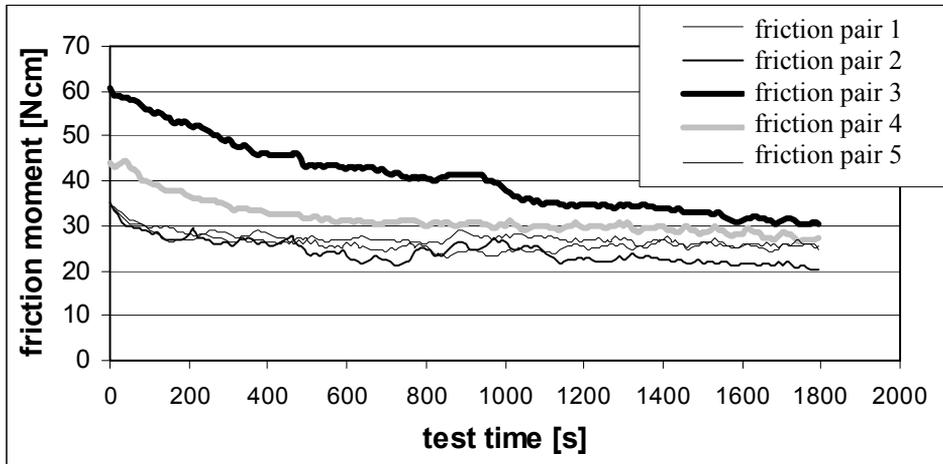
Fig. 2. The course of changes of the friction moment  $M_t = f(t)$  for applied rollers of Class 10
