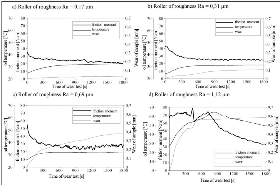
Fig. 5. The comparison of research test results for selected friction pairs, for which rollers of various roughness classes were used
