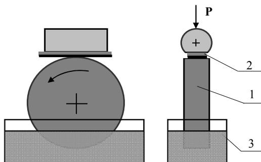
Fig. 1. Accepted configuration of the tested joint: 1 – sample of steel 40HM, 2 – sample of bearing alloy, 3 – engine oil
