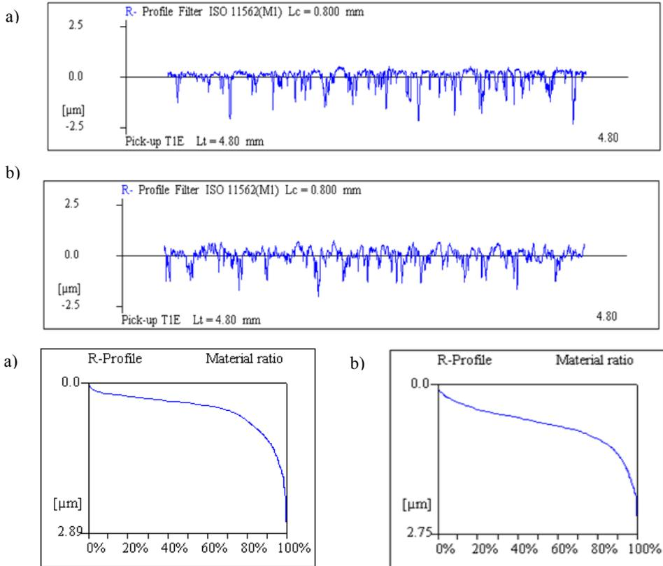
Fig. 3. Comparison of roughness profiles and material ratios of surfaces of selected rollers:
