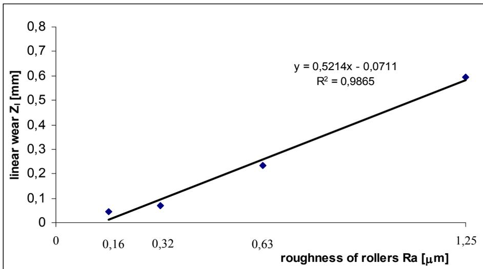
Fig. 4. The relationship between the measure of wear of the samples and average values of roller roughness surface –  $Ra$
