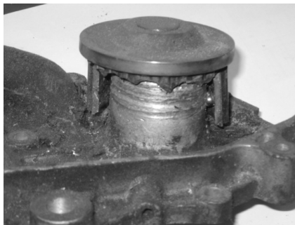
Fig. 8. Total, secondary destruction of water pump (car engine) due to primary bearing failure
