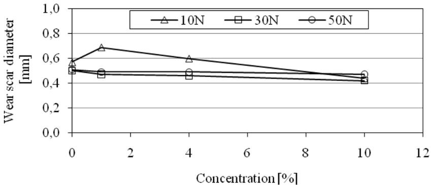
Fig. 6. Dependence of wear scar diameter on concentration of aqueous solutions of Bis-PEG/PPG-20/20 Dimethicone. Tribological test, T-11 testing apparatus, steel ball - steel disc couple, test duration 900 s, sliding velocity 0.1 m/s, radius 10 mm, loads 10, 30 and 50 N
