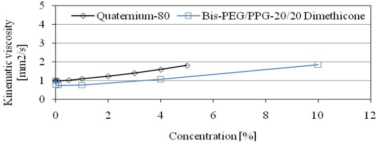
Fig. 2. Dependence of kinematic viscosity on concentration of aqueous solutions of Quaternium-80 and Bis-PEG/PPG-20/20 Dimethicone
