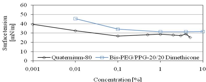
Fig. 1. Dependence of surface tension on concentration of aqueous solutions of Quaternium-80 and Bis-PEG/PPG-20/20 Dimethicone. The value of surface tension for water is about 72 mN/m
