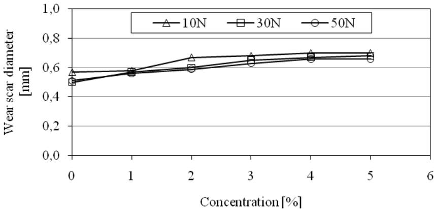
Fig. 5. Dependence of wear scar diameter on concentration of aqueous solutions of Quaternium-80. Tribological test, T-11 testing apparatus, steel ball-steel disc couple, test duration 900 s, sliding velocity 0.1 m/s, radius 10 mm, loads 10, 30 and 50 N
