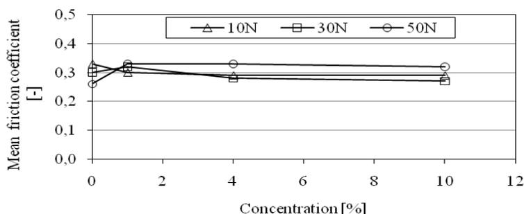
Fig. 4. Dependence of mean friction coefficient on concentration of aqueous solutions of Bis-PEG/PPG-20/20 Dimethicone. Tribological test, T-11 testing apparatus, steel ball-steel disc couple, test duration 900 s, sliding velocity 0.1 m/s, radius 10 mm, loads 10, 30 and 50 N
