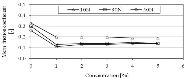
Fig. 3. Dependence of mean friction coefficient on concentration of aqueous solutions of Quaternium-80. Tribological test, T-11 testing apparatus, steel ball-steel disc couple, test duration 900 s, sliding velocity 0.1 m/s, radius 10 mm, loads 10, 30 and 50 N
