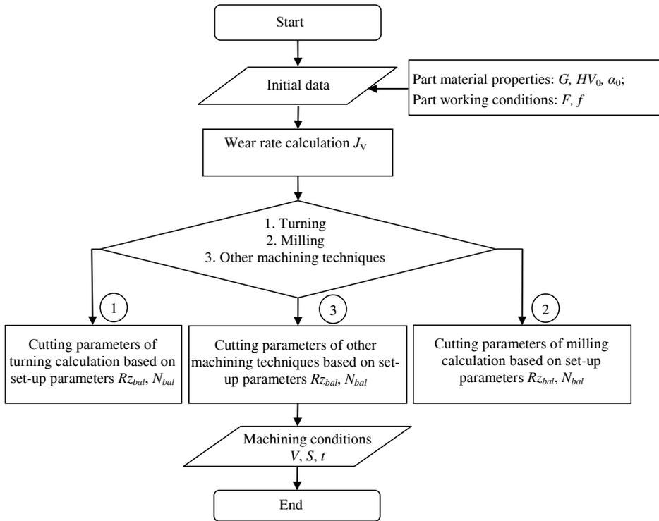
Fig. 1. Algorithm of machining condition calculations of machine components surface layer wear resistance
