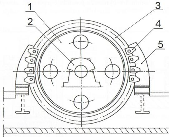
Fig. 1. Multi-rope friction sheaf hoist with hydraulic disc brake system, where: 1 – multi-rope drum, 2 – journal bearing, 3 – brake disc connected to the drum, 4 – hydraulic brake calliper, 5 – callipers stand
