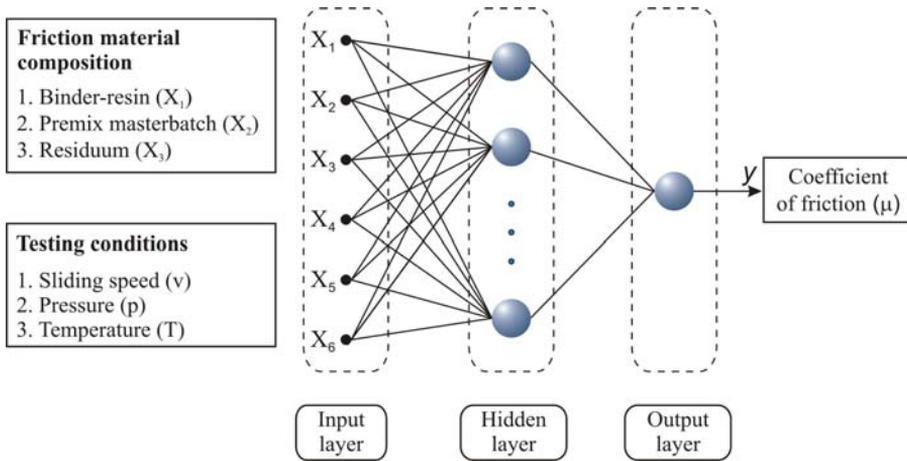
Fig. 3. Structure of the ANN type FFBP used for friction modelling process
