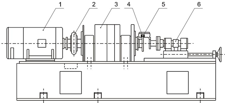
Fig. 2. Schematic diagram of scaled-down inertia dynamometer, where: 1 – electric motor, 2 – flexible coupling, 3 – flywheel, 4 – brake disc, 5 – specimens holder, 6 – torquemeter
