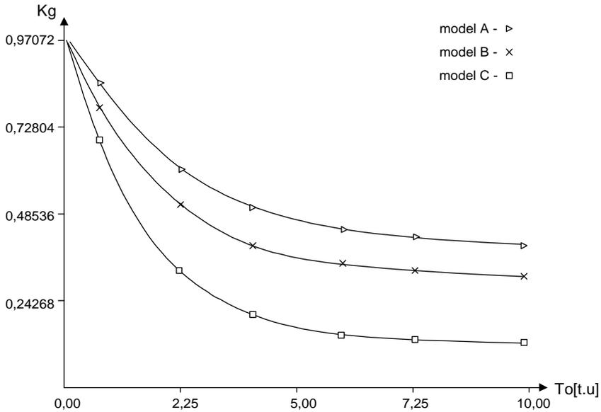
Fig. 7. Availability function  $K_g(t)$  of operation process models tested (for linear functions of expenditures) for  $T/T_a = 2$  and  $N/T_o = 1$
