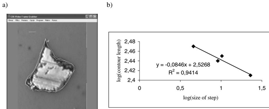
Fig. 5. The determination of the fractal dimension of the scuffing wear particles under a contact load of 500 N. The particle with marked break line (a) and regression line for relation  $\log[L(x)]$  and  $\log x$  (b)
