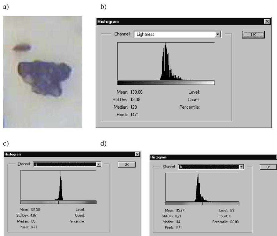
Fig. 2. Image of a fatigue wear particle under contact load of 100 N (a) and histograms of grey levels (b) and components a (c) and b (d)
