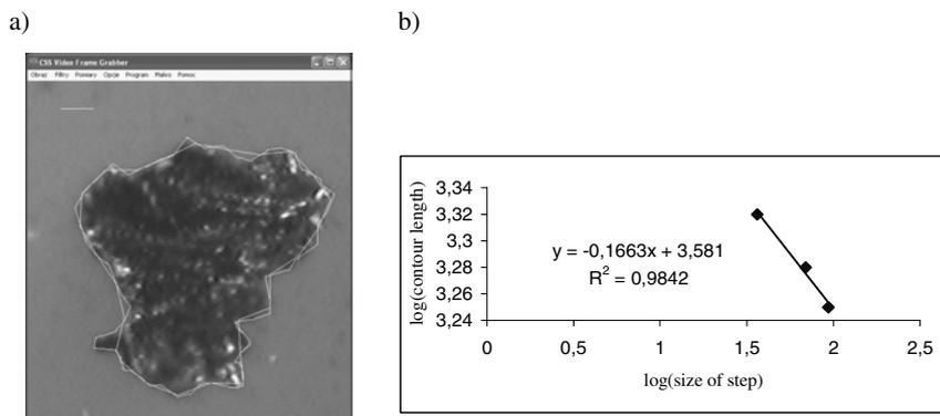
Fig. 6. The determination of the fractal dimension of the scuffing wear particles under a contact load of 1000 N. The particle with marked break line (a) and regression line for relation  $\log[L(x)]$  and  $\log x$  (b)
