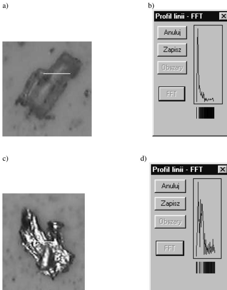
Fig. 3. Images of the adhesive wear particles under contact load of 10 (a) and 50 N (c) and correspond to them Fourier amplitude spectra (b) and (d)
