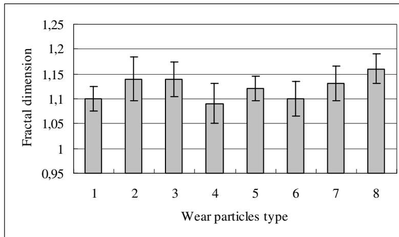
Fig. 7. The graph of the average values of the fractal dimension for the investigated types of the wear particles: adhesion under load of 10 N (1), 30 N (2), 50 N (3), scuffing under load of 500 N (4), 1000 N (5), abrasion (6) and fatigue under load of 50 N (7) and 100 N (8)
