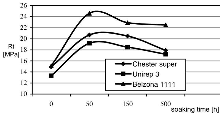
Fig. 2. Joints on shearing durability changes under the long-lasting influence of raised temperature (100°C) [3]
