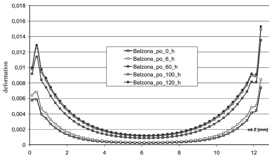
Fig.12. Non-dilatational strain ( $\gamma_{zy}$ ) along adhesive joint for Belzona 111 change in time
