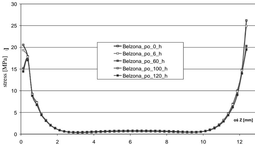
Fig.11. Critical main stresses along adhesive joint for Belzona 111 change in time
