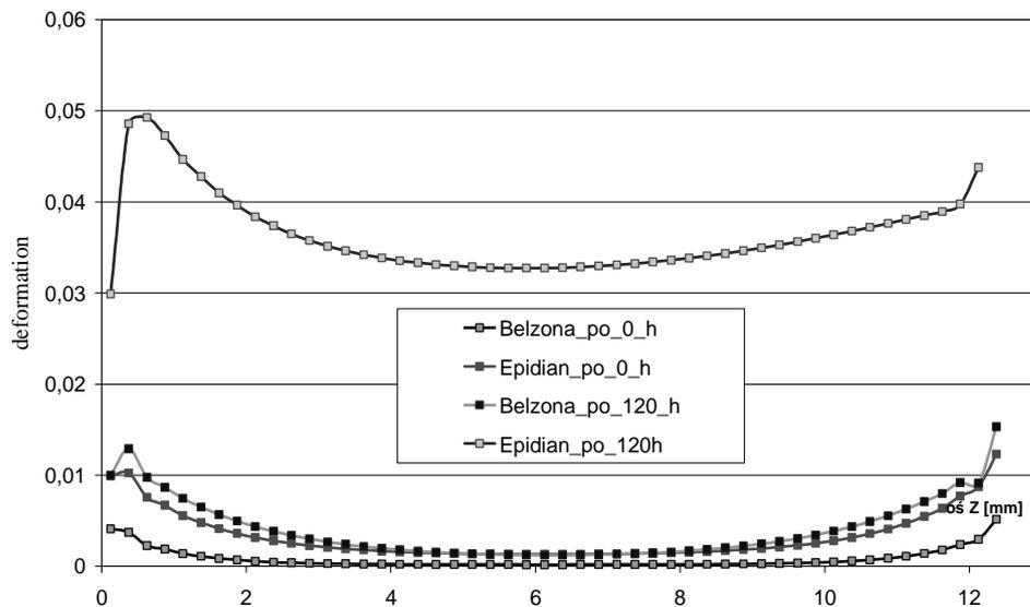
Fig. 14. Maximal principal strains change of time, along adhesive-bonded joint for two adhesive models (Epidian 57 and Belzona 111) at time of imposing load and after 120 h simulated time
