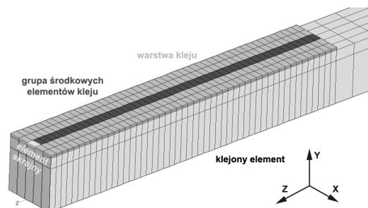
Fig. 9. Overlapping joint numeric model with the middle elements group and extreme element marked
