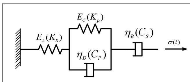
Fig. 3. Adhesive-bonded joint physical proprieties model, used for creeping phenomenon calculation in NASTRAN program
