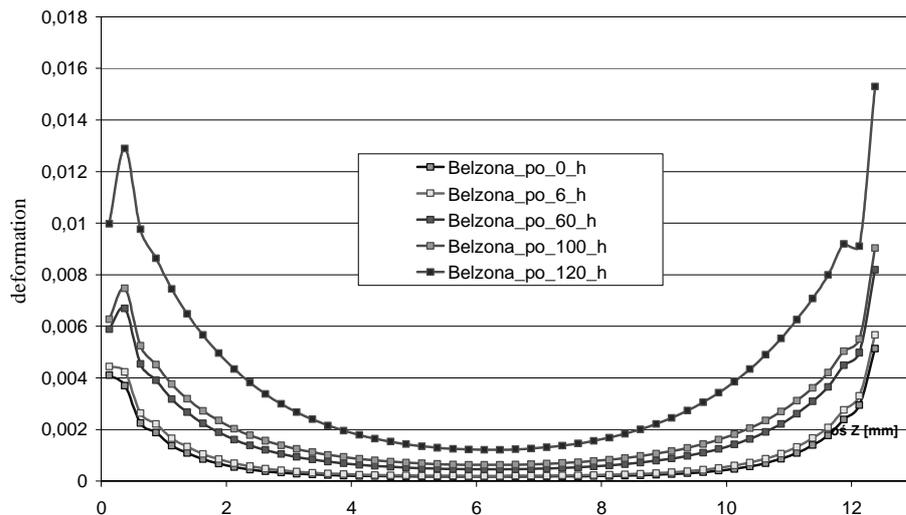
Fig. 13. Critical main strain along adhesive joint for Belzona 111 change in time
