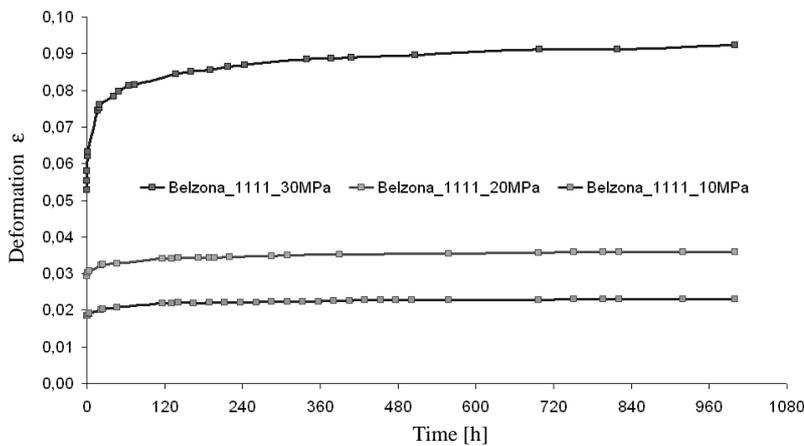
Fig. 5. Belzona 1111 composite creep curves formulated for different stresses at 60°C
