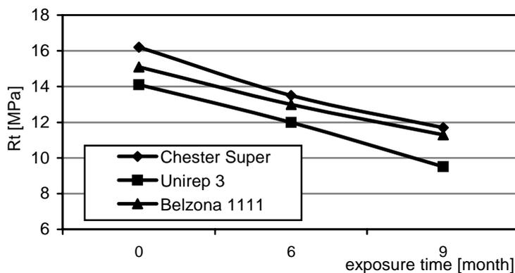
Fig. 1. Aged joints on shearing durability changes in natural conditions [1]
