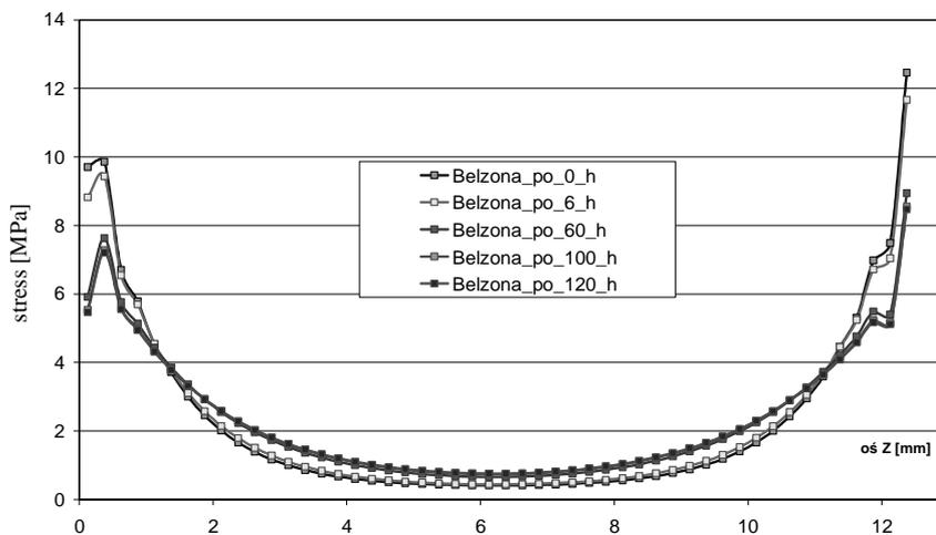
Fig.10. Shearing stresses ( $\tau_{zy}$ ) along adhesive joint change in time
