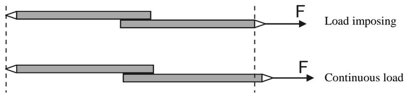
Fig. 8. Scheme of the two-staged load of overlapping specimen
