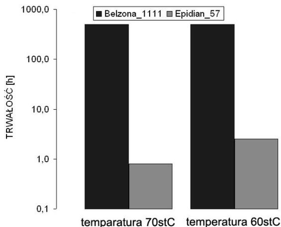
Fig.15. Durability of joints tested under load of 0,6Pn at 70°C and 60°C
