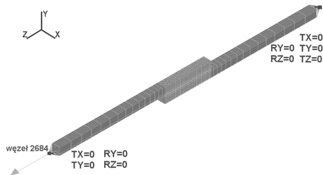
Fig. 7. Method and place of supporting and loading of adhesive joint
