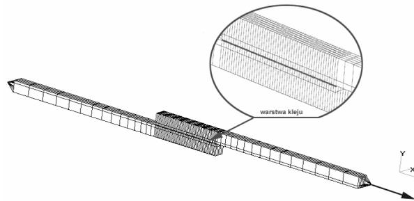
Fig. 6. Discrete model of shearing load overlapping adhesive joint
